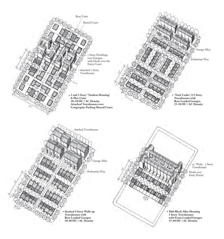
A simpler pattern, which achieves the same density but replaces townhouses with flats, involves arranging three stories of stacked walk-up flats around a pair of stairs, one facing the street, the other giving access to surface parking at the rear. Each flat thus has a double aspect, facing both the street and the rear of the site. With a 25-ft.-wide frontage, there is also enough room for each flat to be designed with side-by-side rooms.
